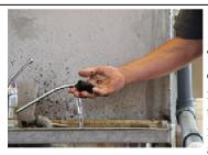
This picture shows checking coagulation or flocculation to monitor polymer dosage. When the water runs clear and the solids stay in a ball means you are at the correct polymer dosage.
